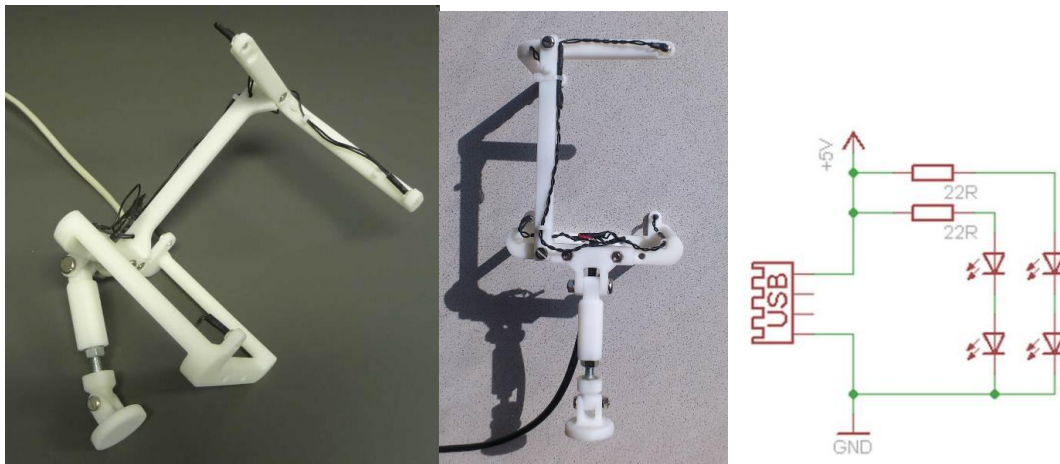
Figure 8: IR-LED frame assembly and schematic
