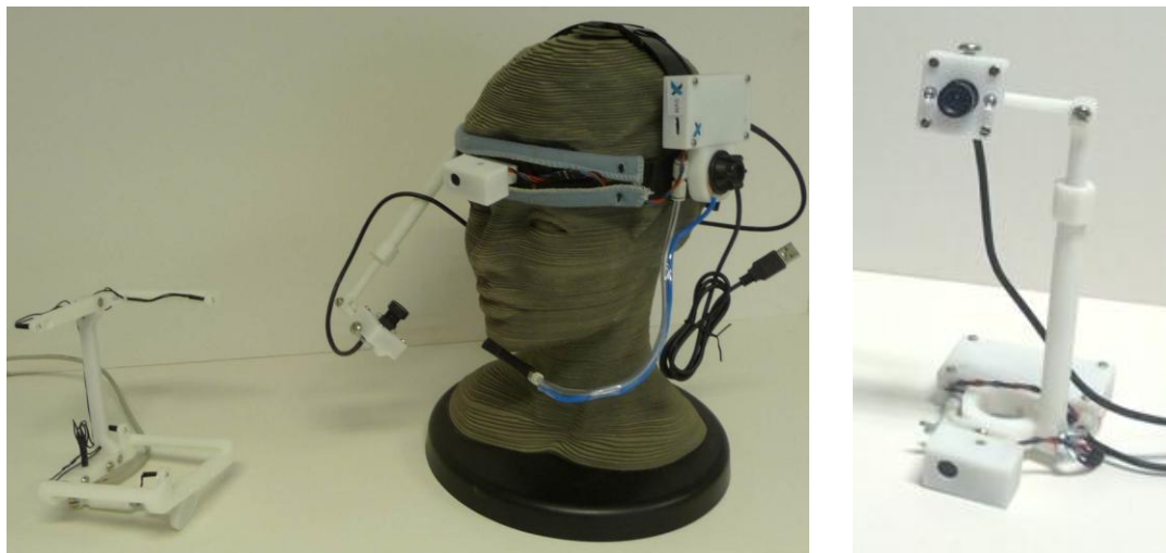
Figure 1: a) Complete SVM for gaze tracking (left), remote blob tracker (right)
