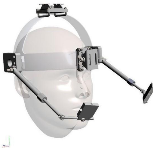
Figure 3: Virtual 3d-model of the AsTeRICS head-mounted SVM support gear
