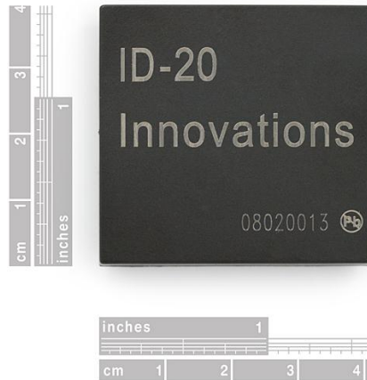
Figure 8: ID-Innovations integrated RFID reader component (here: ID-20)
