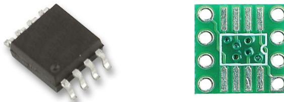
**Figure 3. ADuM3100 digital isolator (left) and Pin SOIC to DIP8 board (right).**
