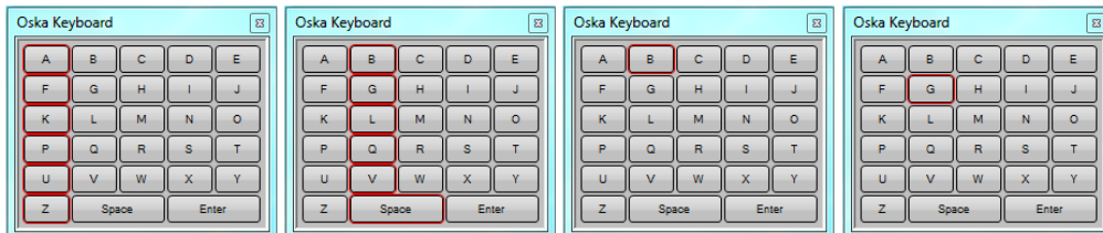
Figure 47: Column-row scanning in Oksa keyboard
