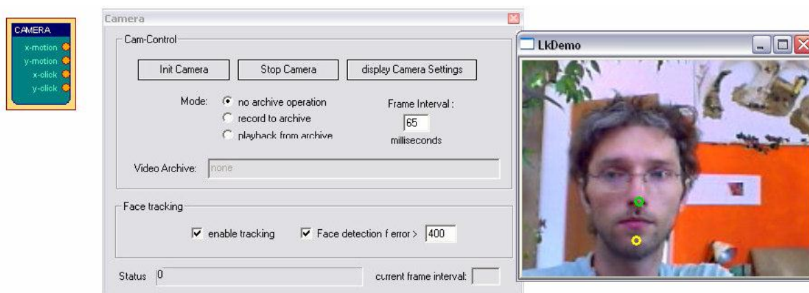
Figure 128: BrainBay camera element properties, live camera view with feature detection
