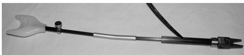
Figure 59: The prototype of the pneumatic gripper equipped mouthstick [3]
