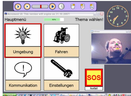
Figure 130: Using the Autonomy environmental control system via BrainBay camera mouse
