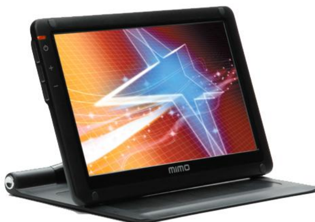
Figure 4: MIMO 720-S USB pluggable LC display with touchscreen
