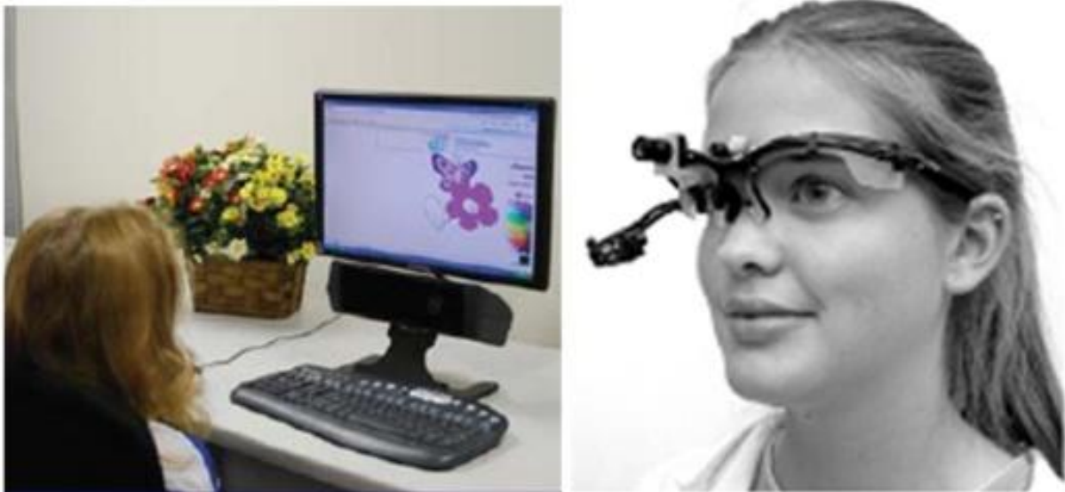
Gaze tracker: wearable (head mounted, Rochester Inst.) on the left and remote on the right.
